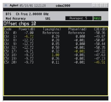
\*Meas Setup: Advanced/Multi Channel Estimator = ON
