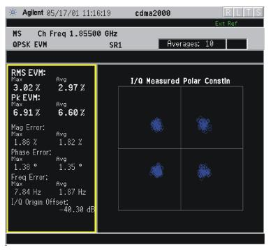
**Step 9.** Press the View/Trace, I/Q Error (Quad View) keys to display a combination view of the magnitude error, phase error, and EVM graph windows, and the modulation summary result window.
