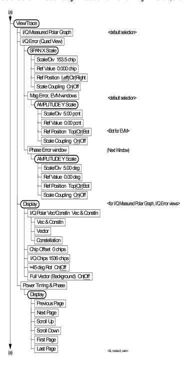
Figure 6-22 Modulation Accuracy Measurement Key Flow (4 of 4)
