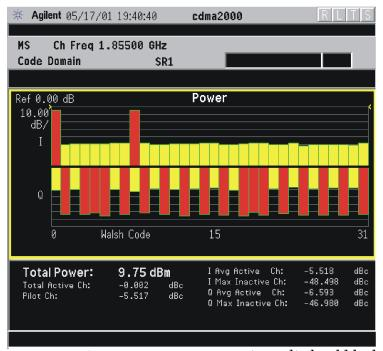
The Code Domain: Power measurement result should look like the above figure. The graph window and a text window is displayed. The text window shows the total power level along with the relative power levels of the various channels.
