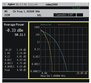
The CCDF measurement result should look like the above figure. The measurement result values are shown in the summary result window.
